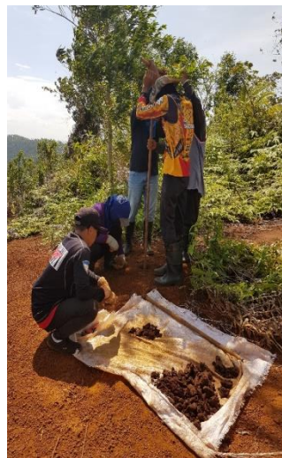
Samples from auger hole PGC_CUA_06 in Barangay Cuarinta, San Jose, PDI with the total depth of 0-4.5 m. GPS Location: N10°00'42.7" E125°36'10.7"
