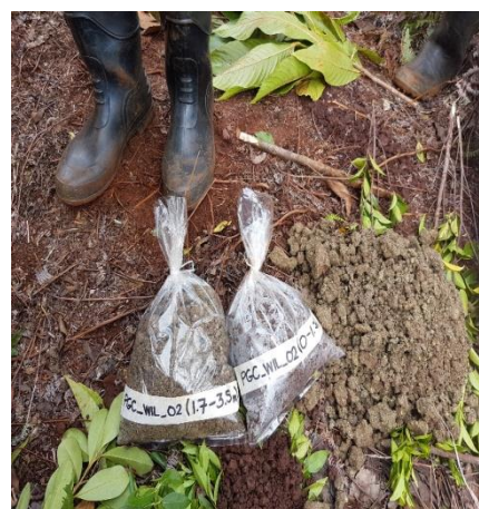
Samples from auger hole PGC_WIL_O2 in Barangay Wilson, San Jose, PDI with the total depth of 0-3.5 m. GPS Location: N10°02'20.3" E125°35'09.1"
