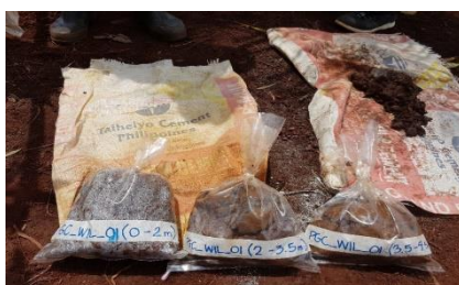
Samples from auger hole PGC_WIL_O1 in Barangay Wilson, San Jose, PDI with the total depth of 0-4.5 m. GPS Location: N10°02'20.7" E125°35'11.9"
