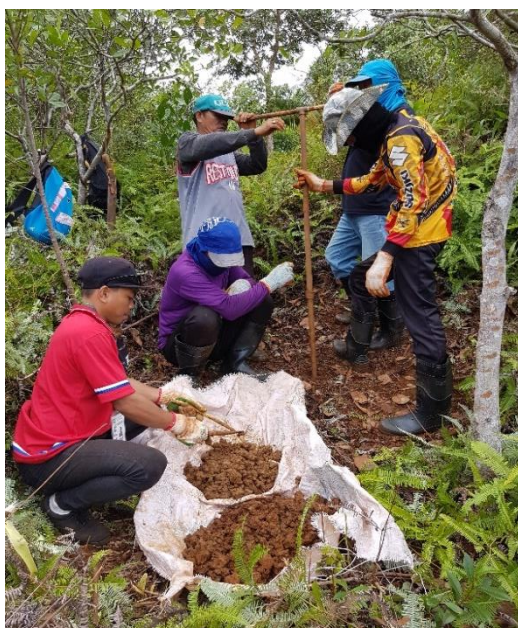
Samples from auger hole PGC_CUA_O4 in Barangay Cuarinta, San Jose, PDI with the total depth of 0-4.5 m. GPS Location: N10°00'50.0" E125°36'10.2"
