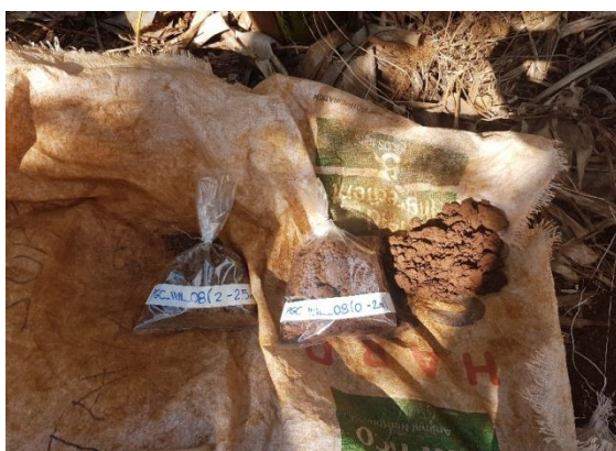
Samples from auger hole PGC_WIL_08 in Barangay Wilson, San Jose, PDI with the total depth of 0-2.5 m. GPS Location: N10°01'52.6" E125°35'34.2"
