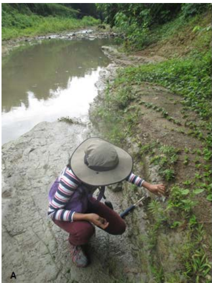
(A) Acid test performed in determining the calcareous content of the outcrop located at Agol Creek, Brgy. Santo Cristo. (B) strike and dip of the outcrop is N 53^{\circ} E and 9^{\circ} SE, respectively. (GPS Location: N 13^{\circ} 05' 29.4'' , E 123^{\circ} 30' 15.1'' )
